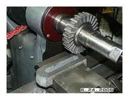
With one clean surface the others are now milled using this as a reference and always working against it. Since everything is tapered the clamping becomes problematic. By using a rod I have a single plane to push against the reference and to mill the sides. (Figure 2) The part was then rotated and the bottom was milled.
