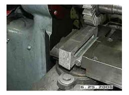
At this point, the method of clamping was changed to the setup shown in figure 3 and the third side was machined. You may consider this a rough machining process because I still needed to get the width of the fingers correct.
