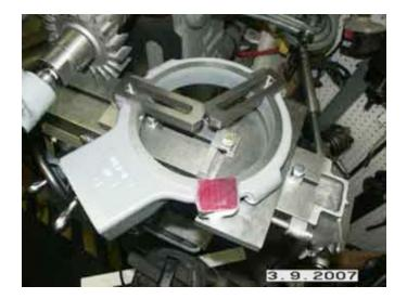
The assembly was then rotated 120 degrees with the large mounting boss still to the outside and the third slot was cut using the same procedure.
