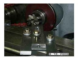
The beveling process turned out fine except that on the last finger there was a hard spot in the casting and I got a shower of sparks and messed up the end mill good.
