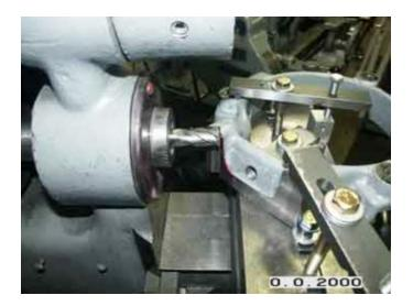
Next a vee-groove needed to be cut for the prismatic way. Paula showed how to do it on a vertical mill. The horizontal mill let me clamp the large casting in a safer manner. While I do have a 90-degree cutter for the over arm/arbor mode of the mill I was unable to figure out a method of securing the base half of the steady rest. I chose instead to tilt the base at 45 degrees and use an end mill while moving the knee up this is shown in above.
