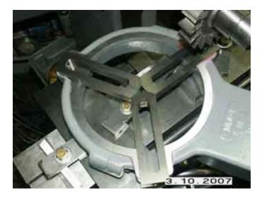
Next the excess of the mounting foot was cut off. The casting is sized for use on either a 10" or 9" lathe. You are given a dimension and cautioned the "Your mileage may very", measure your own lathe. Yeah! That's not a trivial measurement. I tried and come up with a number about 0.015 under the "target" dimension. I cut it to my measurement, Should have left it alone.
