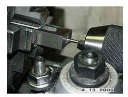
Well, I thought they were on-center, I managed to get two of the fingers 0.100 off center. No problem for facing but I drilled two holes 0.100 off center. I fixed this by making cast iron plugs from some of the scrap I cut off on the band saw and press fitting the plugs in the misplaced holes and re-drilling the holes. If you notice, the pictures have dates on them; this program is now extending over several months and it will be several more months until it's finished.
