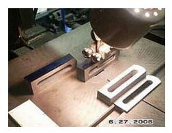
Yes that is a wood cutting band saw! I have a 10-14 tpi metal cutting blade in it and I have replaced the singlephase motor 1750 RPM with a 3 Phase 1150 RPM motor and a VFD. Running at about 15 Hz I get a speed that's fine for metal. Turning the VFD up to 90 Hz puts me back at 1750 RPM and that's fine for wood. Yes I have used a metal blade for wood and it works fine. It just slices through metal like butter.
