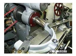
While I was in this setup, the boss for securing the steady rest to the lathe was faced and drilled. Since I wanted to use the same wrench for the steady rest as for the tailstock the hole was opened to 15/32. I did have to come back later and tale about 1/8 off the web just below the hole so the wrench would have enough clearance. (Figure 13).
