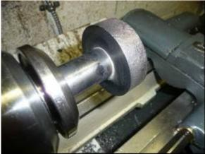
Figure 3: Facing rear of mount bushing. \*\*\*
