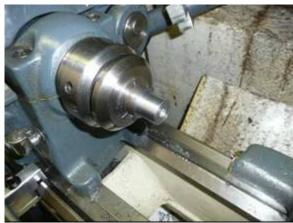
Figure 2: Turning 1" drill rod.
