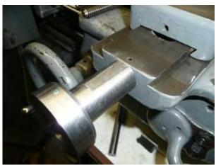
Figure 15 The finished extension sleeve with markings and flat. \*\*\*
