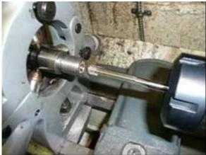
Figure 10 Stub removed, bushing pressed, faced, and reamed.
