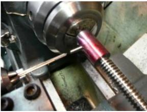
Figure 21: Drill, ream and install taper pin \*\*\*
