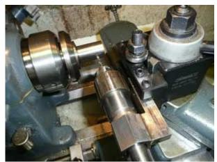
Figure 17: Cross drilling weep hole \*\*\*
