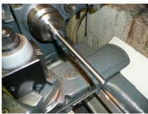
Figure 18: 3/8 rod aligned and pressed \*\*\*
