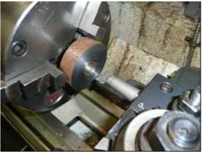
Figure 1: Boring 0.875 for the 1" rod.
