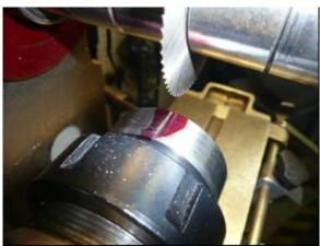
Figure 13 Marking the zero reference line \*\*\*
