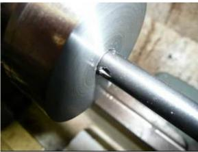
Figure 4: Boring ID to insure concentricity.
