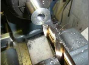
Figure 16: Drilling for dial and handle shaft insert \*\*\*
