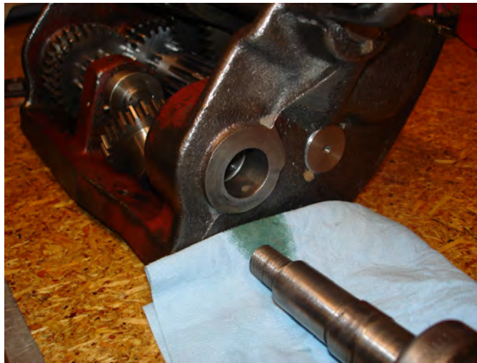
Figure 146: Reinstalling the leadscrew in the gearbox.
