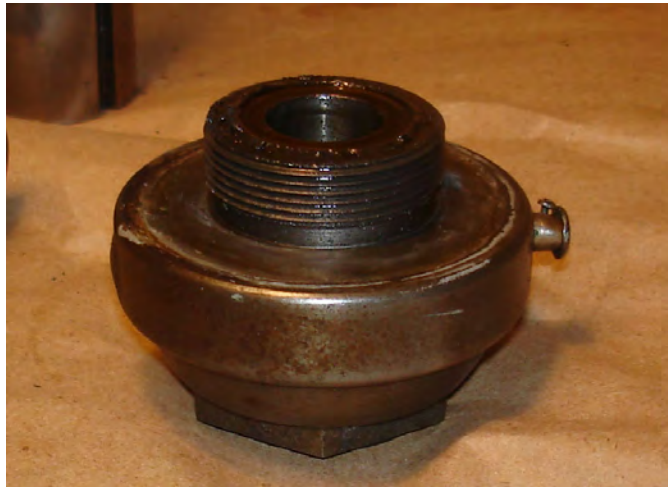
Figure 194: Tailstock rear bushing removed.
