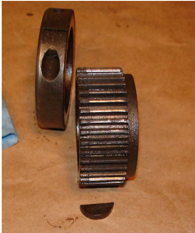
Figure 41: Takeup nut gear and key.
