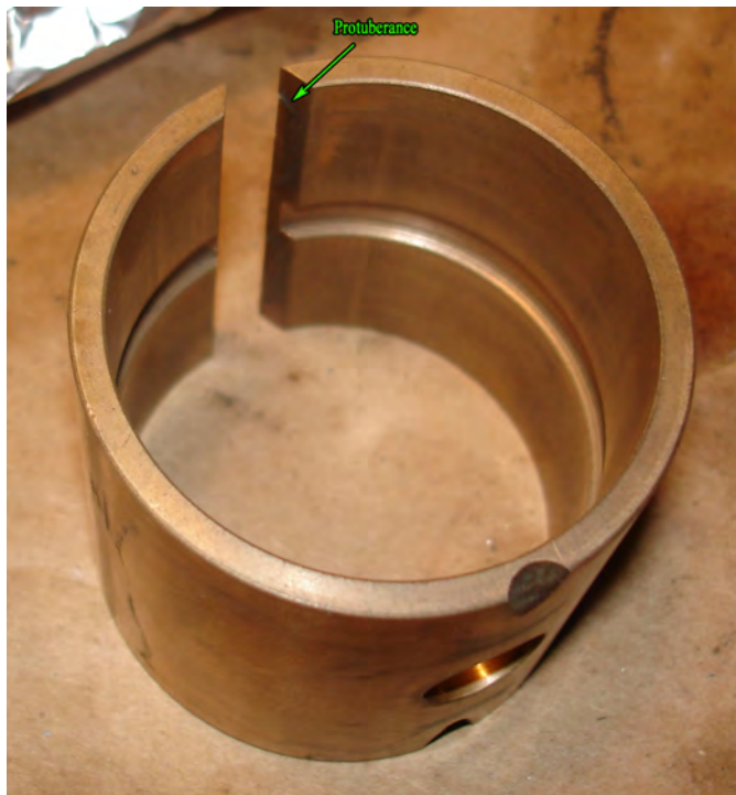
Figure 52: Cleaned rear bearing showing where expander has damaged the bearing by being reinstalled on top of the slot rather than in it.
