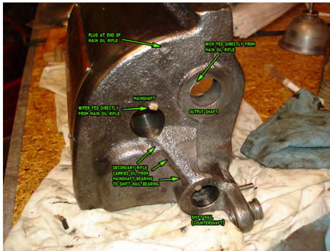
Figure 139: Side of gearbox showing lubrication points.
