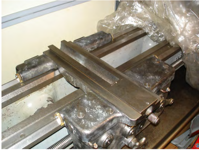
Figure 191: Saddle cleaned and reinstalled.
