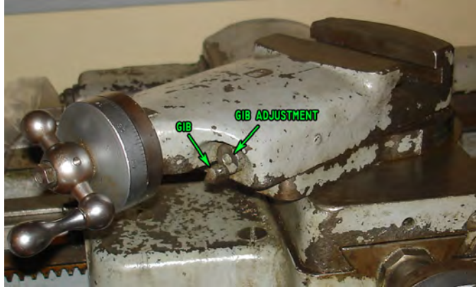
Figure 108: Compound rest gib adjuster.
