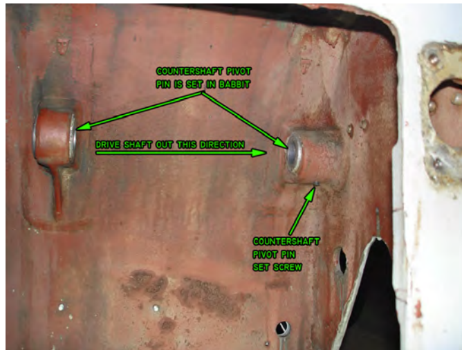
Figure 5: Showing location of countershaft pivot set screw.
