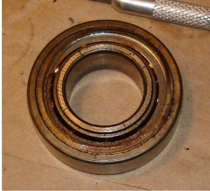
Figure 16: Original countershaft bearing with shield removed.
