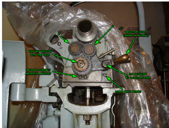
Figure 62: Reversing gear train prior to removal.
