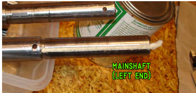
Figure 141: Mainshaft showing new felt.
