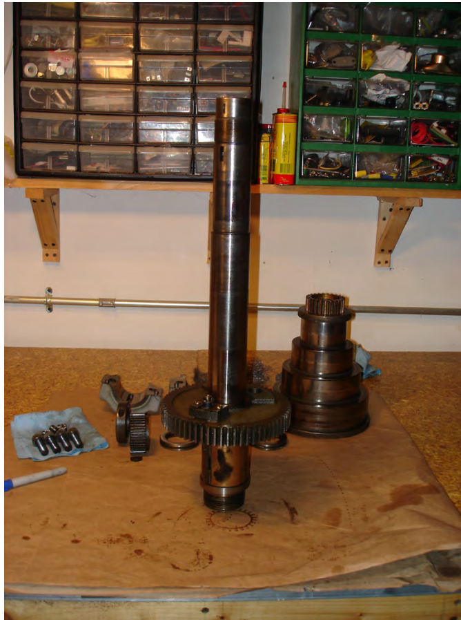
Figure 44: Overview of spindle with pulley cone removed.
