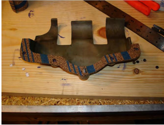
Figure 183: New sump gasket in position.
