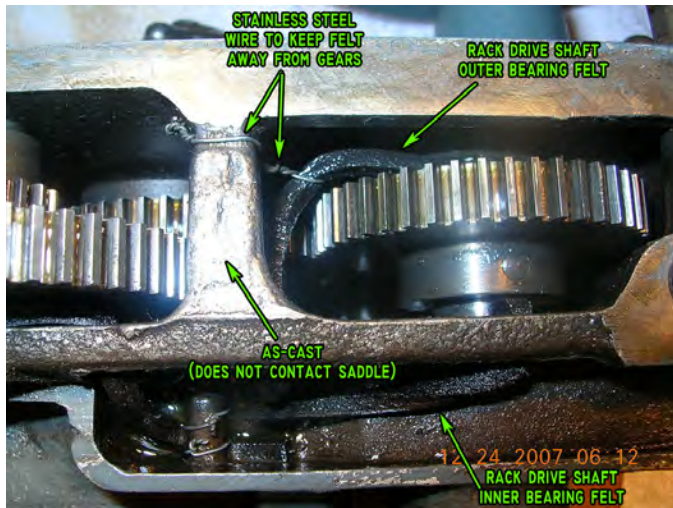
Figure 171: A heavy 10 apron showing different upper felt routing.
