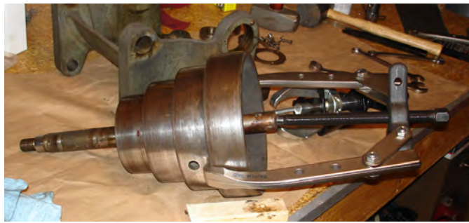
Figure 14: Pulley has been removed from the casting and is being pulled off the shaft.
