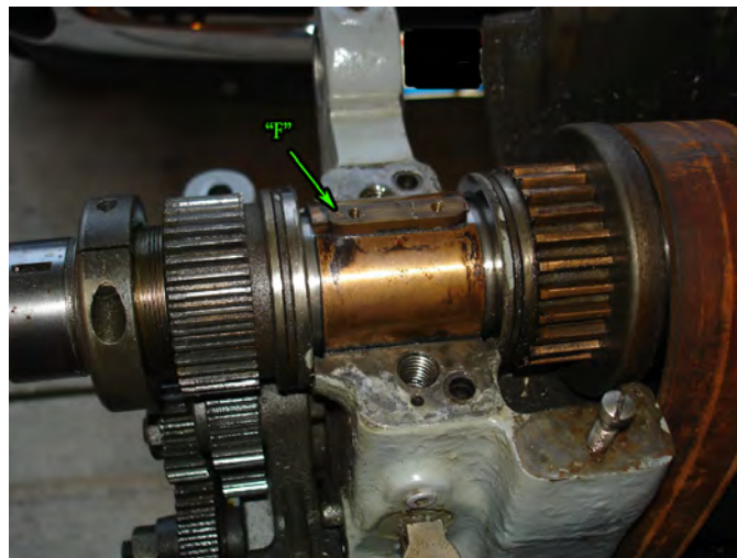
Figure 40: Rear bearing cap removed. Notice the "F" indicates this expander is in the wrong orientation.
