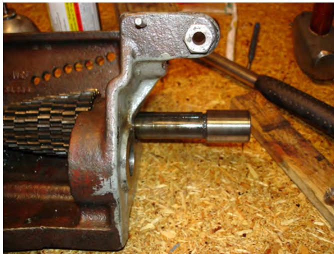
Figure 134: Mainshaft being removed.
