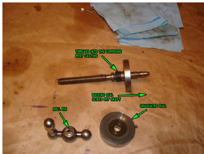
Figure 106: Parts of the compound rest dial.
