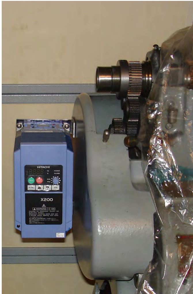
Figure 100: One VFD mounting option.
