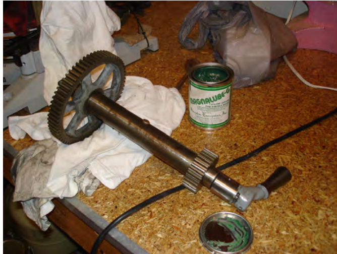
Figure 36: Cleaned and assembled back gear.
