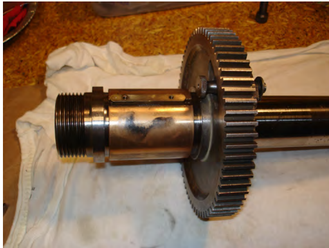
Figure 58: Bull gear installed.
