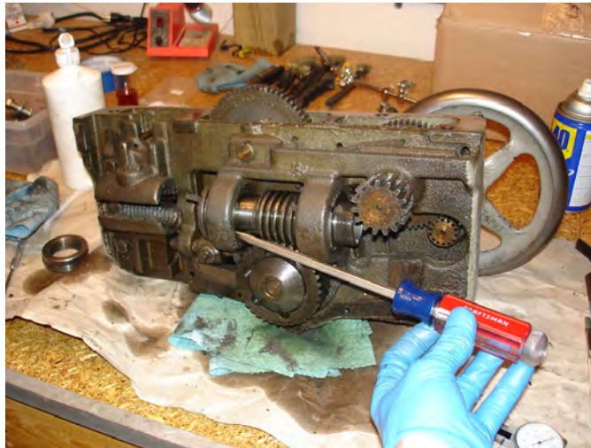
Figure 156: Driving out the worm drive end caps.
