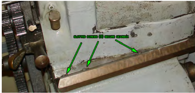
Figure 123: Screws that secure the gearbox to the bed.
