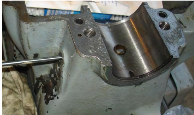
Figure 61: Wick retention rod.
