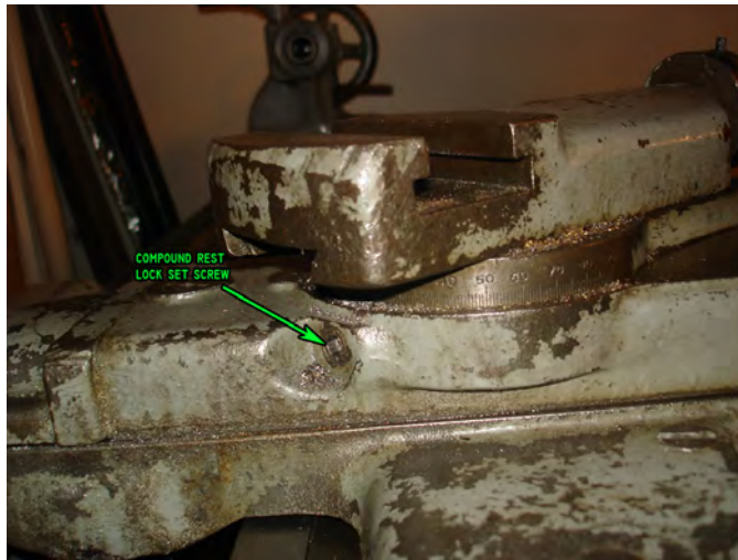
Figure 102: Compound rest lock screw. There is a second one on the other side.
