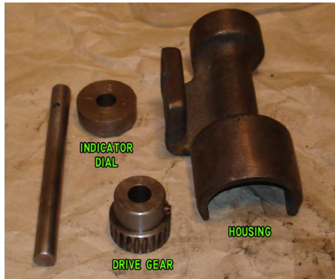
Figure 148: Thread dial parts.
