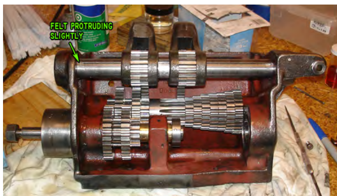
Figure 145: Gearbox showing felt protruding from shift rail.
