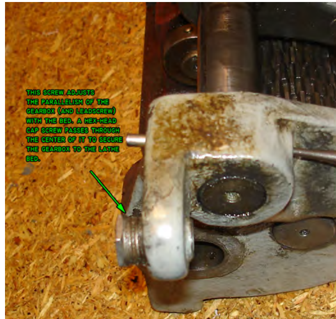
Figure 125: Gearbox parallelism adjuster.
