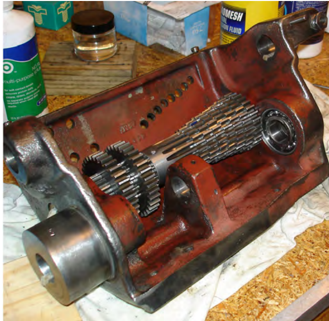
Figure 142: Completed mainshaft installation.
