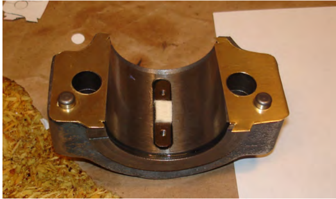
Figure 83: Refurbished rear bearing cap with new expander felt and shims.
