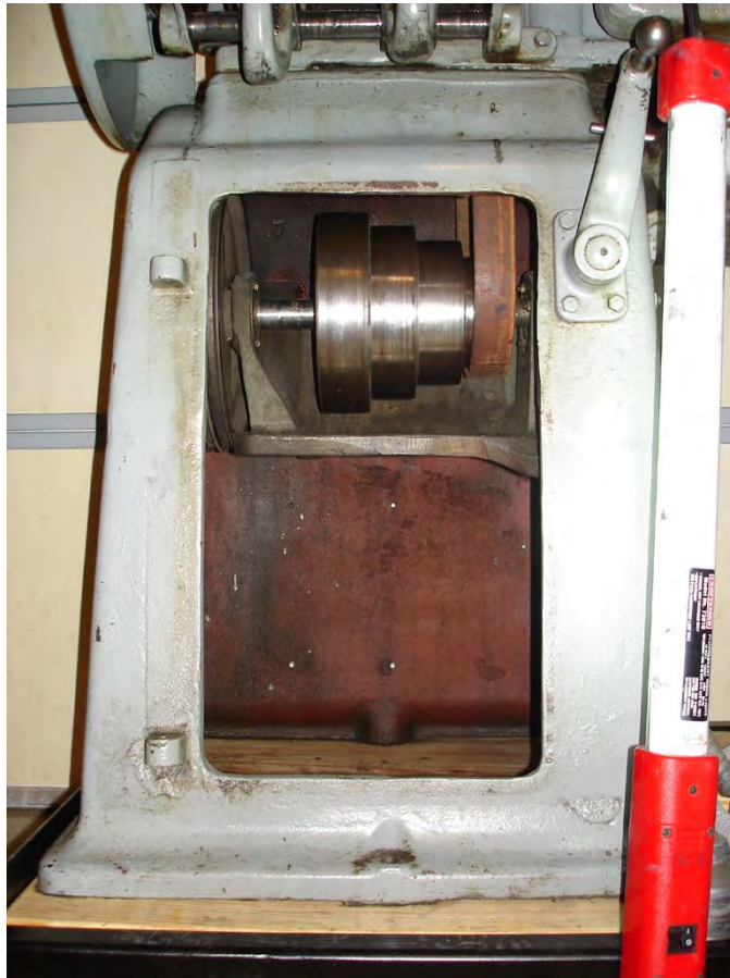
Figure 4: Underdrive after cleaning
