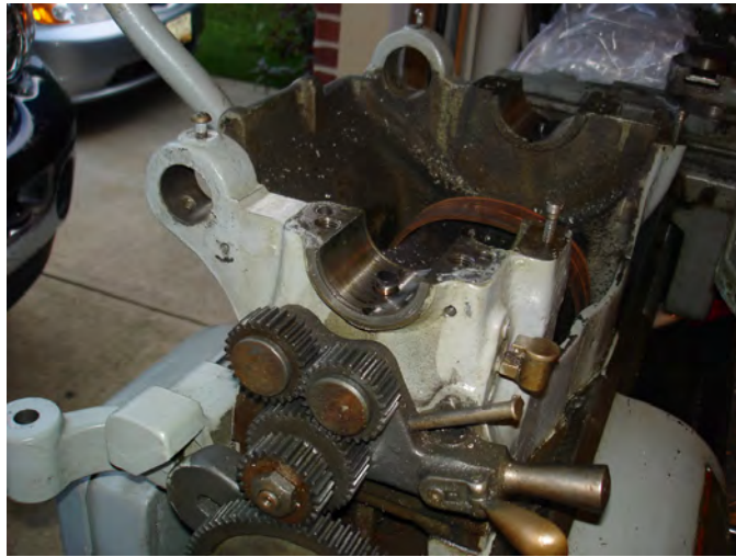
Figure 72: Overview of headstock casting with spindle removed.
