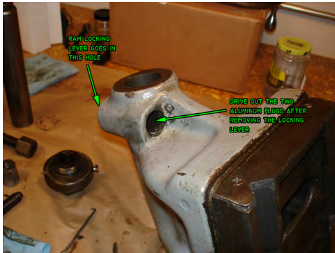
Figure 197: Tailstock ram locking mechanism removed.
