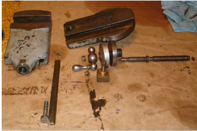
Figure 111: The entire compound rest disassembled.
