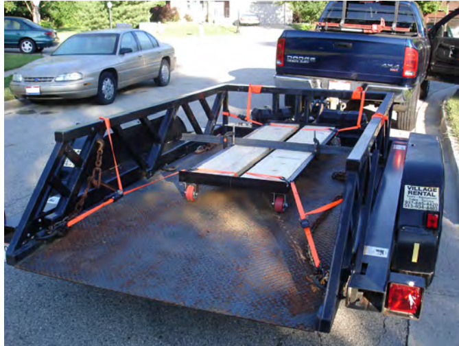
Figure 1: Rolling platform secured to the trailer with straps and ready to depart.
