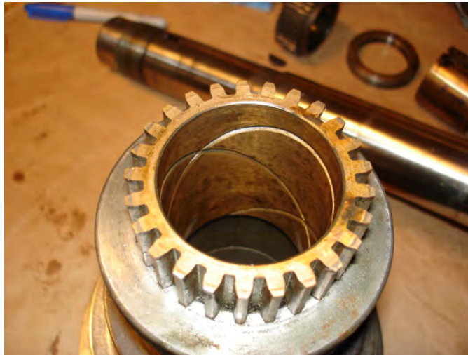
Figure 45: Closeup of rearmost pulley cone bearing.
