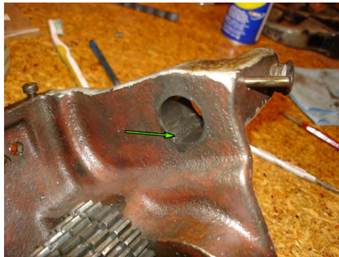
Figure 132: Shift rail hole showing felt wick.
