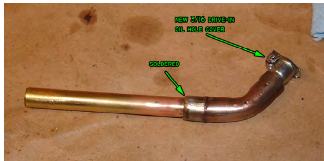
Figure 182: Repaired apron oiler.
