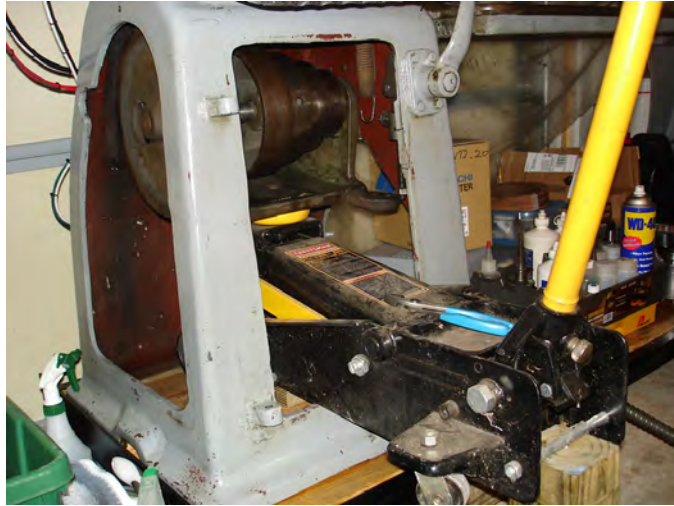
Figure 6: Method for removing the underdrive with a hydraulic floor jack.
