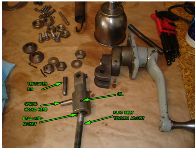
Figure 25: The assembled tensioner to show functionality.
