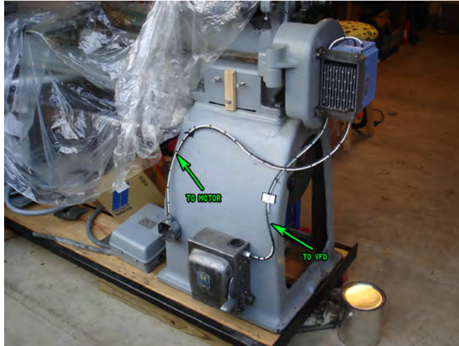
Figure 91: Installed safety switch.
