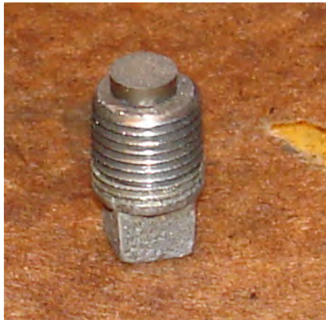
Figure 185: Magnet on apron oil drain plug.
