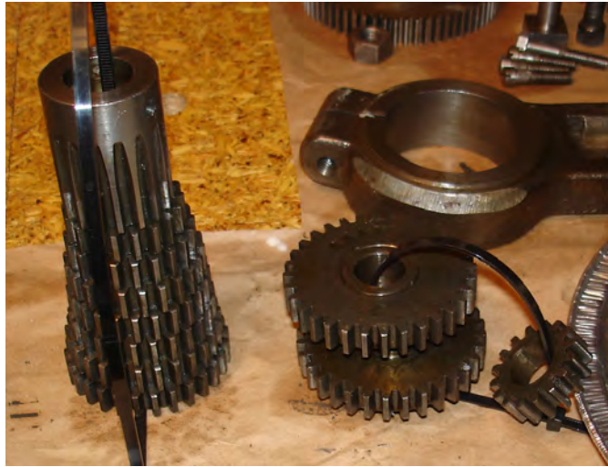
Figure 135: Gears stacked to preserve orientation.
