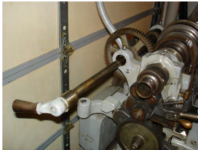
Figure 35: Removing the back gear spindle.
