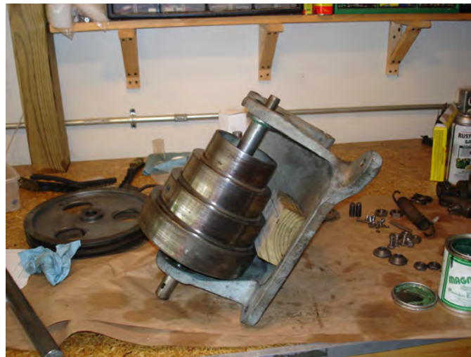
Figure 21: A method for supporting the left end of the countershaft while the right side bearing is pressed into place.
