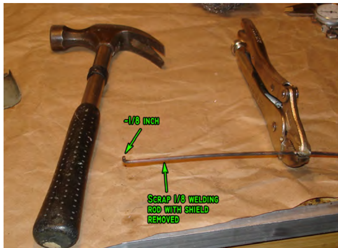
Figure 75: Tool used to extract the oil tube from the front spindle bearing casting.
