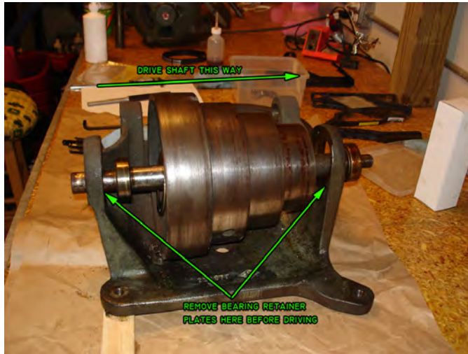
Figure 12: How to remove the underdrive pulley assembly.
