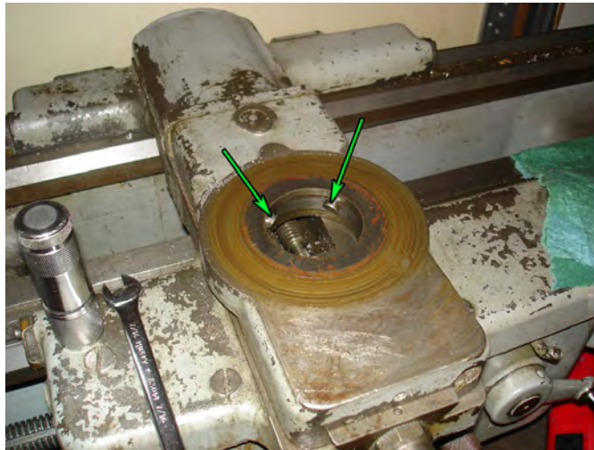
Figure 103: Carriage with compound rest removed.
