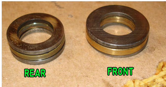
Figure 117: Front and rear cross slide leadscrew bearings.
