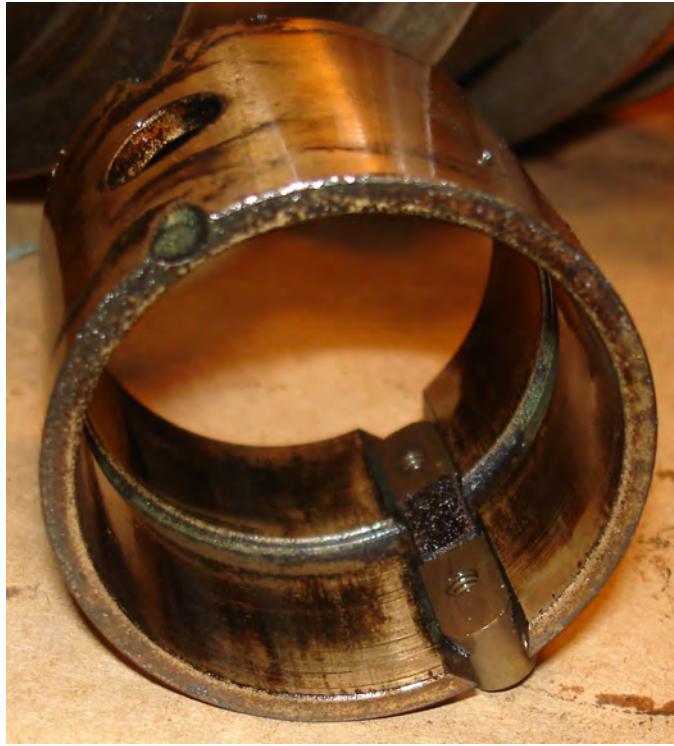
Figure 49: Closeup of rear bearing sleeve.
