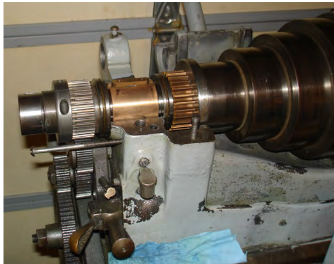
Figure 59: Reinstalled headstock spindle showing rear bearing.
