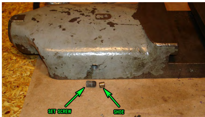
Figure 107: Compound rest gib screw location.
