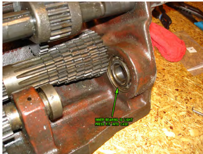
Figure 128: View of inner leadscrew bearing with leadscrew removed.
