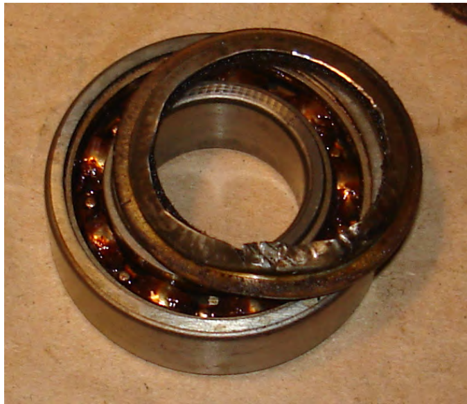
Figure 17: Failed countershaft bearing with shields removed.
