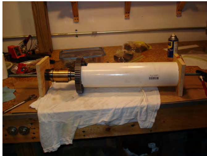
Figure 57: Bull gear being pressed on.
