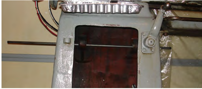
Figure 8: Long punch being used to drive out the underdrive pivot pin.
