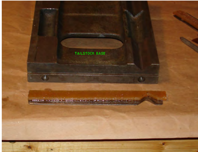
Figure 200: New tailstock base felt.
