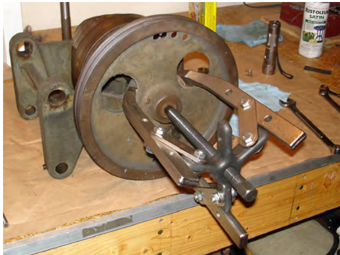
Figure 11: Pulling the vee-belt pulley using a 7-ton OTC brand 2/3-jaw puller.
