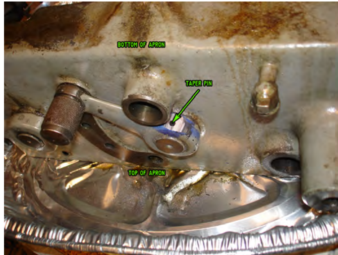
Figure 166: Drive selector taper pin.
