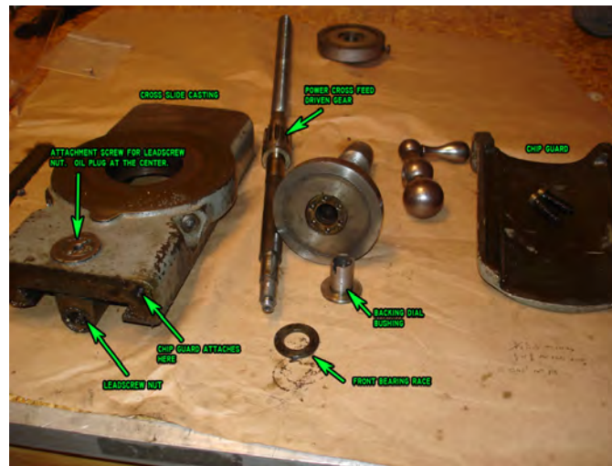
Figure 118: Complete cross slide in pieces.
