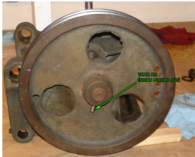
Figure 10: Vee-belt pulley being removed.
