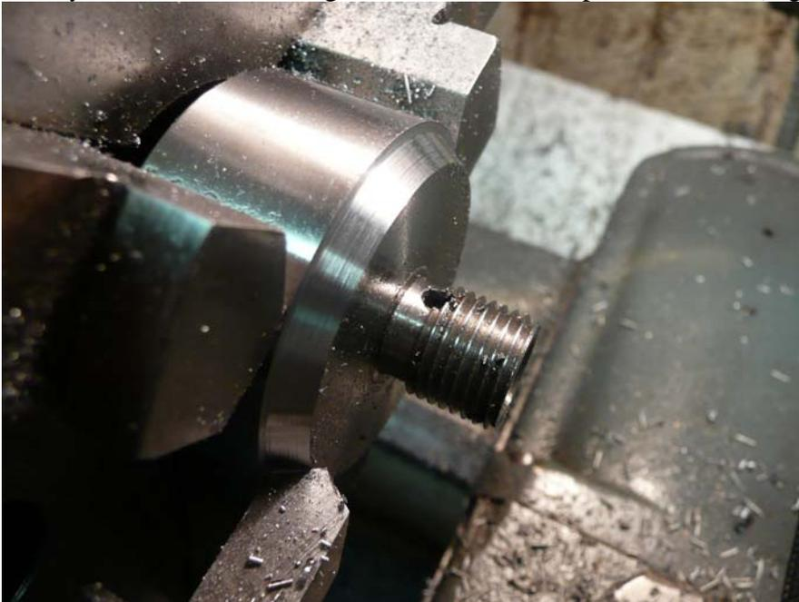
Figure 23 The step on the bevel is there since 1/8" is to be removed from the OD and I wanted the bevel to remain. The same tool was used to put a bevel on the face of the threaded boss.
