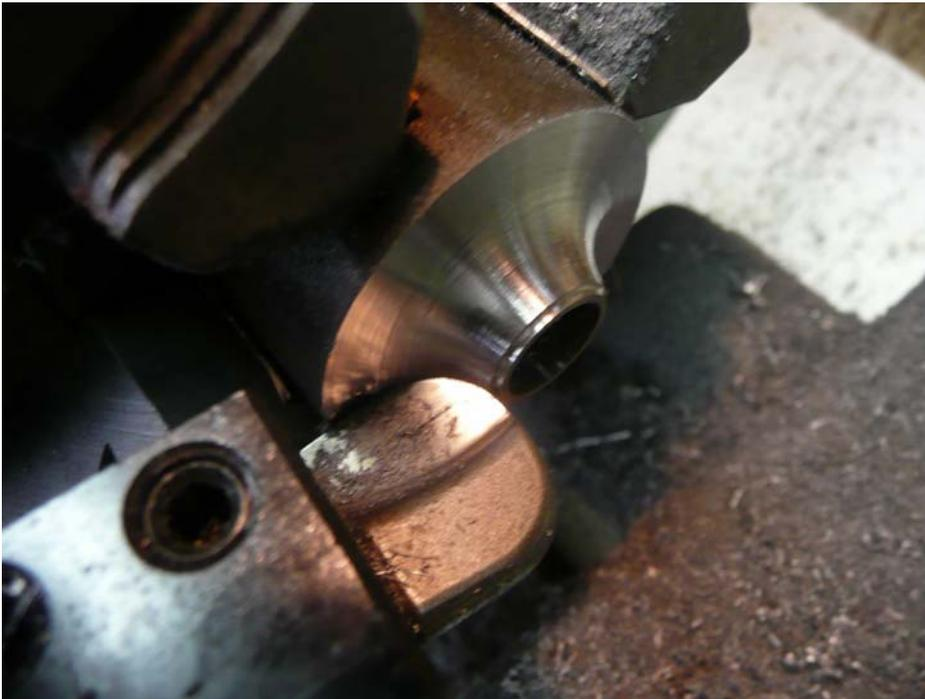
Figure 4 Finishing the machining of the curve with a Router Bit form tool.
