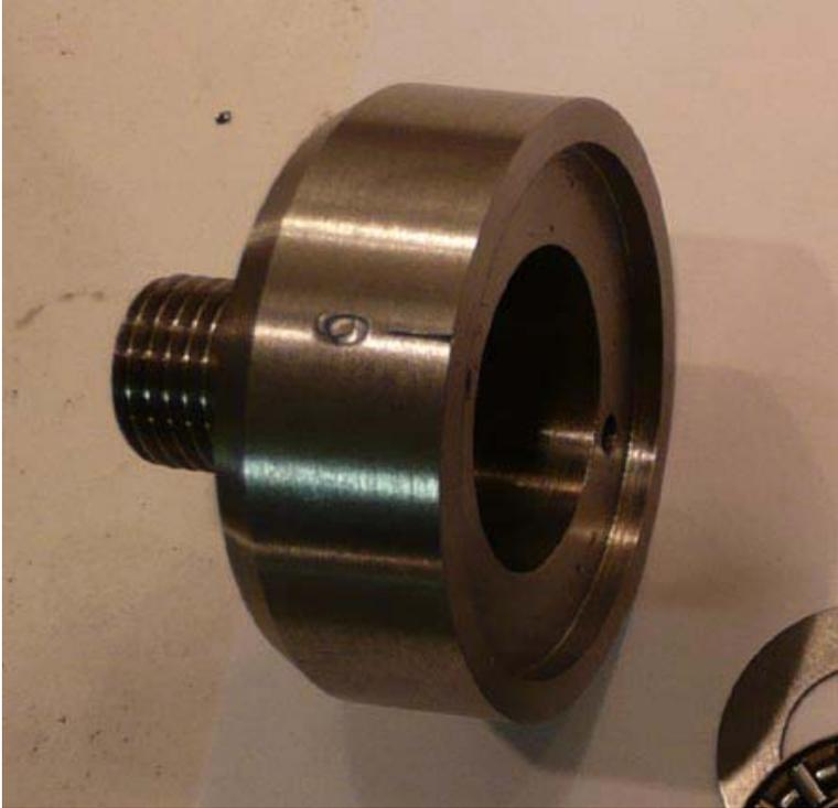
Figure 19 The Bearing Housing.
