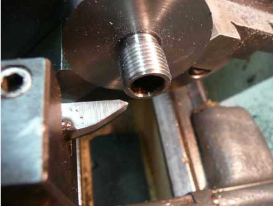
Figure 22 Asymmetric Threading tool
