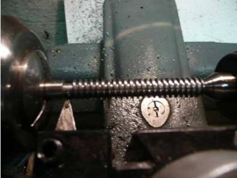
Figure 14 The finished 3/8-10 Acme Screw Blank
