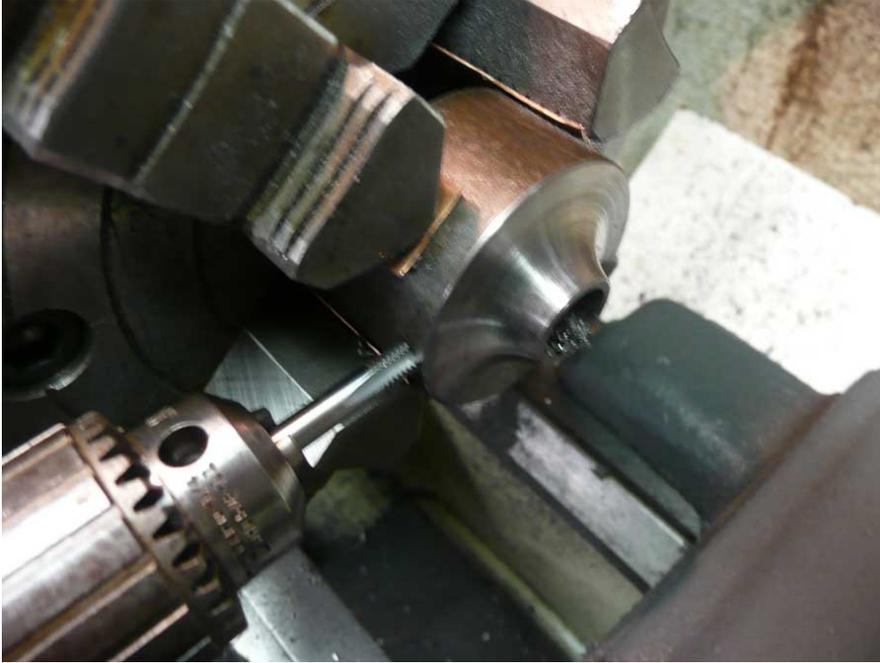
Figure 5 Tapping for the Thumb Screw after cross drilling.
