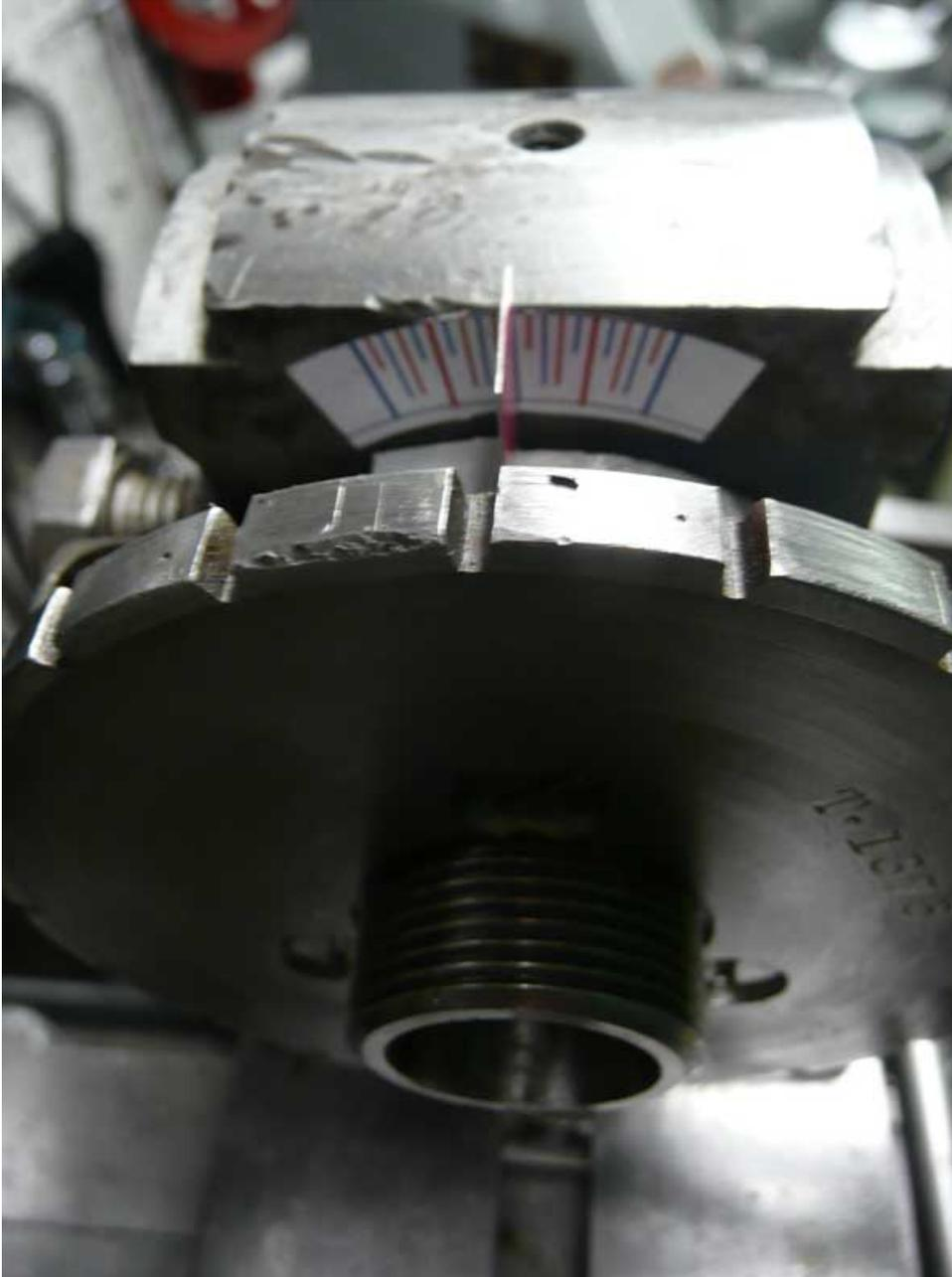
Figure 7 Vernier Scale added to Index Head
