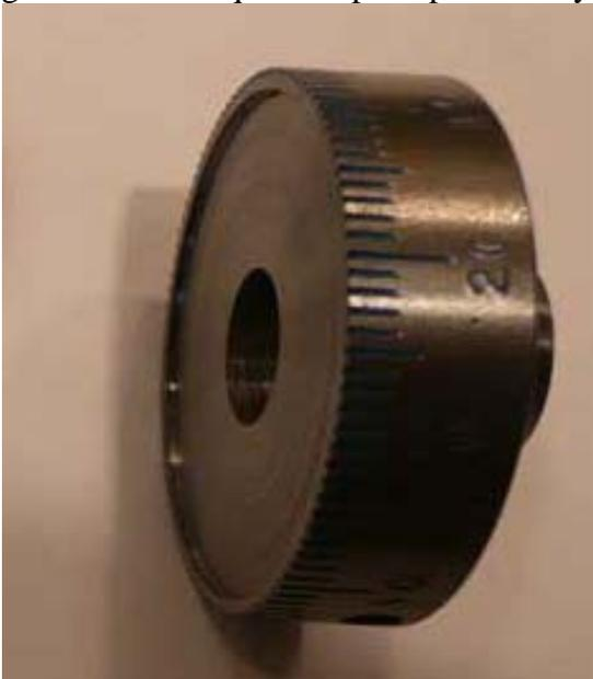
Figure 9 The finished dial with Retainer Ring relief.
