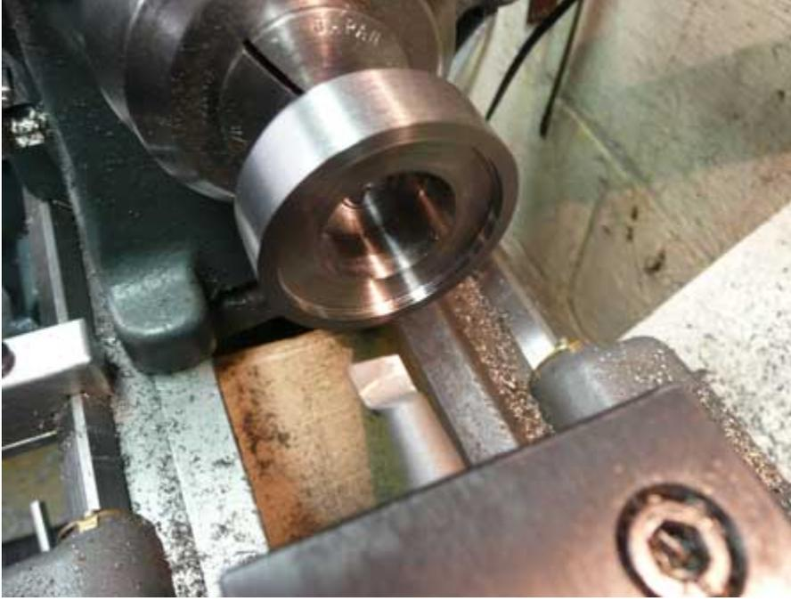
Figure 26 Boring the counter bores in the housing.
