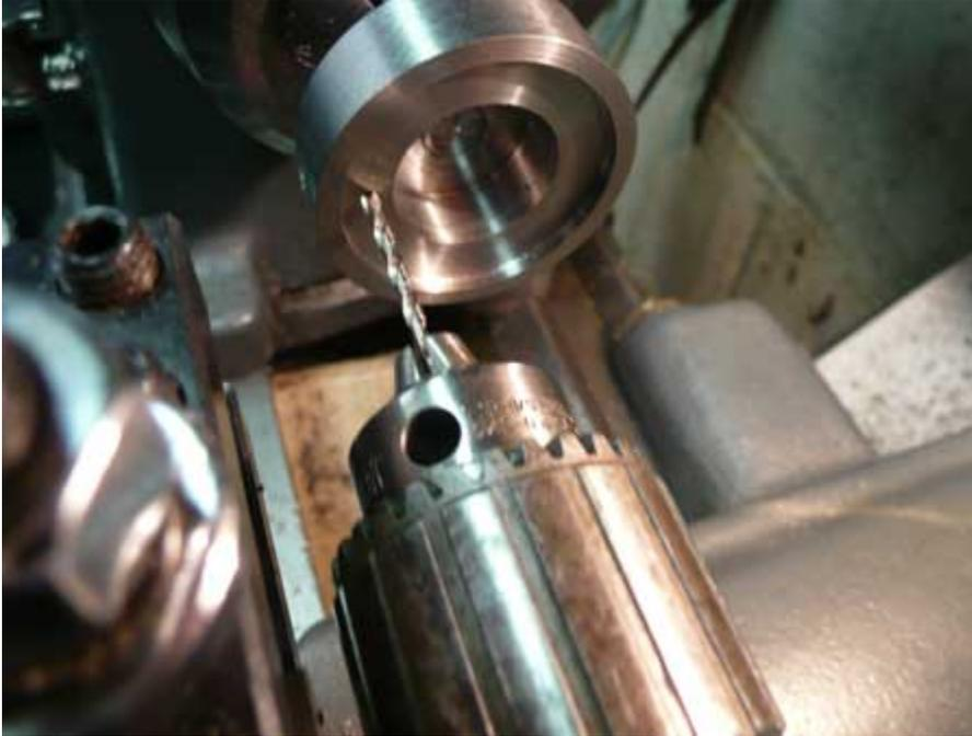
Figure 27 Drilling holes for the Bearing retainer.
