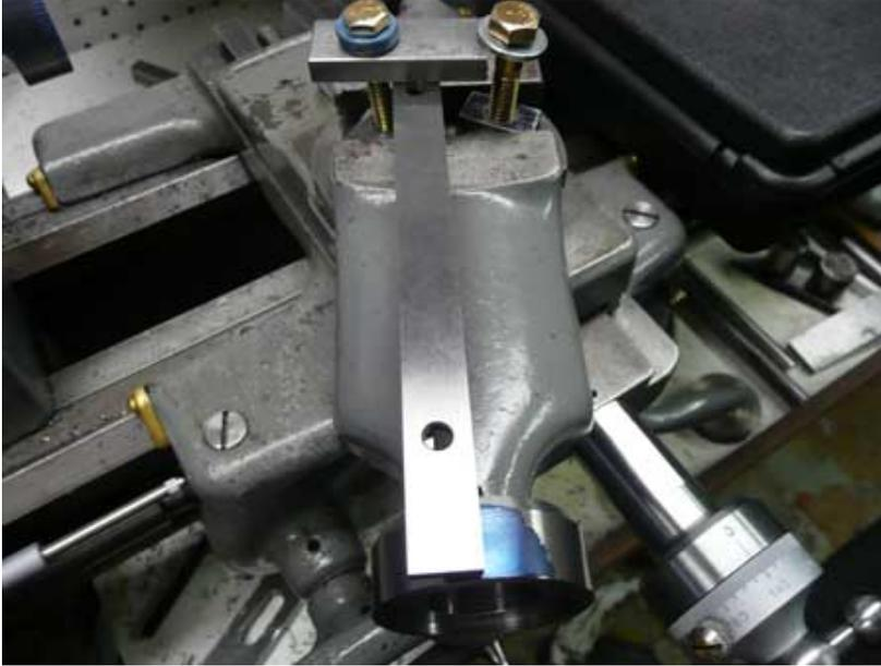
Figure 28 Positioning the Zero Reticule line.
