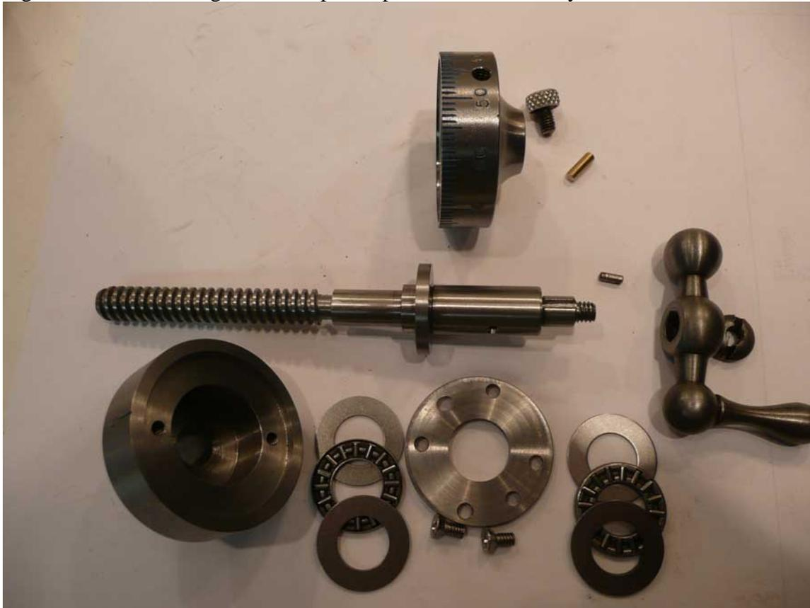
Figure 1 Large Dial Compound Assembly Parts.
