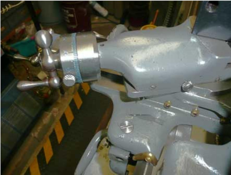
Figure 34 The finished large dial assembly mounted on the compound.
