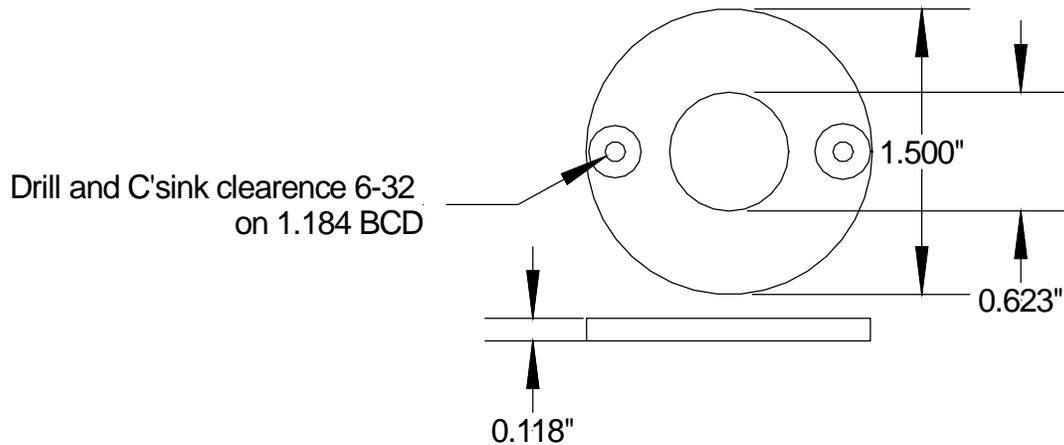
**Figure 30 The Bearing Retainer Ring Dimensions**
