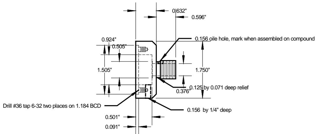
Figure 18 The Bearing and Bushing Housing Dimensions.
