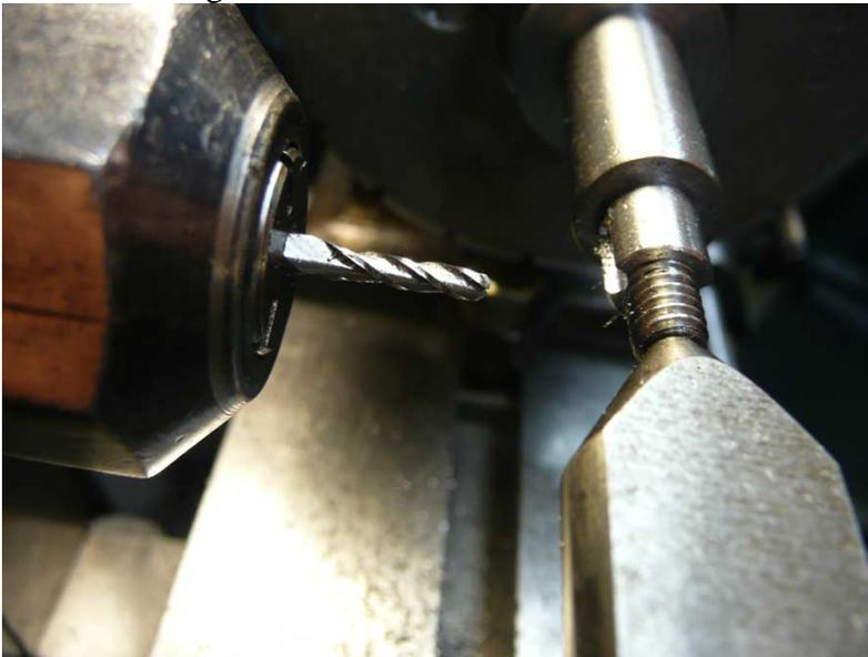
Figure 16 Milling the Key slot.
