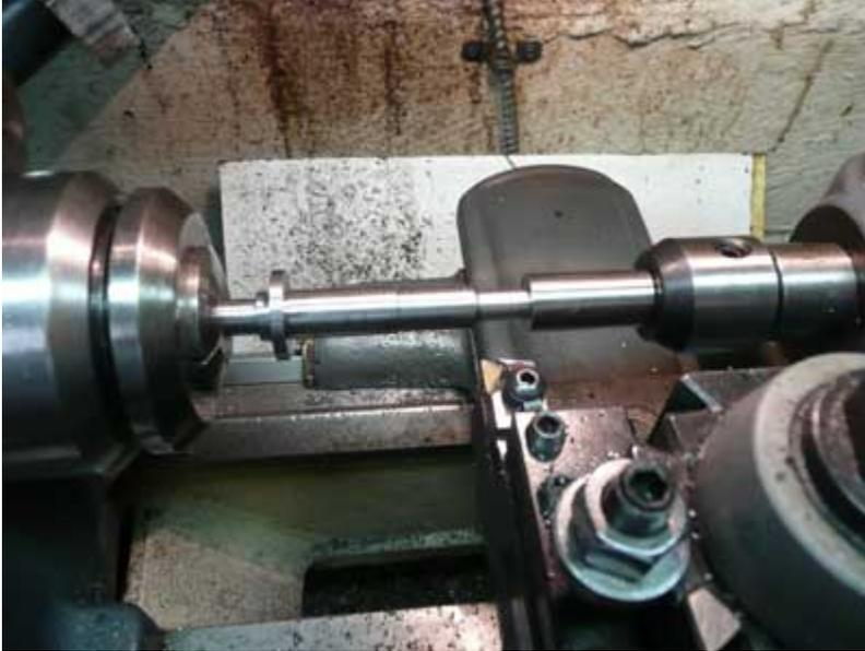
Figure 12 Turning the bearing retainer
