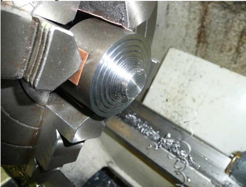
Figure 3 Step approximation to the dial curve.
