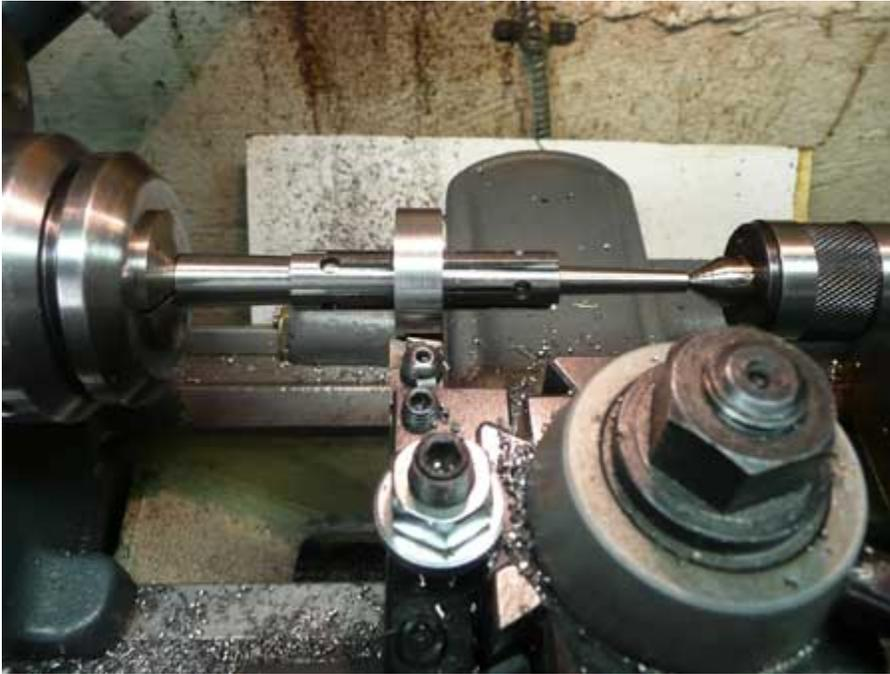
Figure 31 Turning the OD of the bearing retainer.
