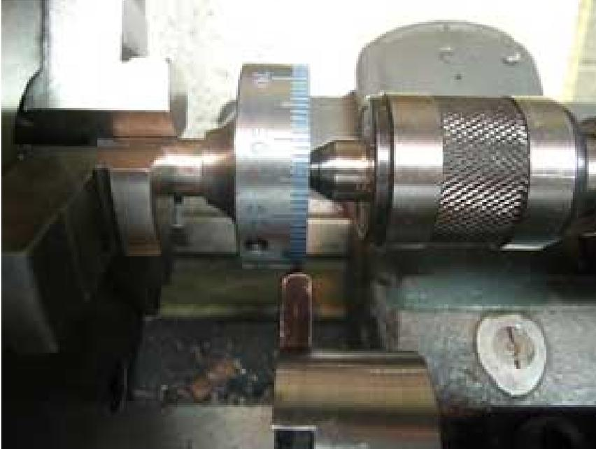
Figure 8 Stamping the numbers on the fabricated dial
