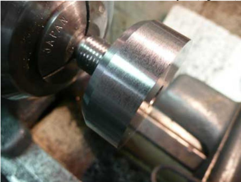
Figure 25 Mounted on the Mandrill, the OD is turned and the part faced to length. The depth of the mandrill must be set careful since several counter bores are to be made and you do not want to have to machine the drill rod.
