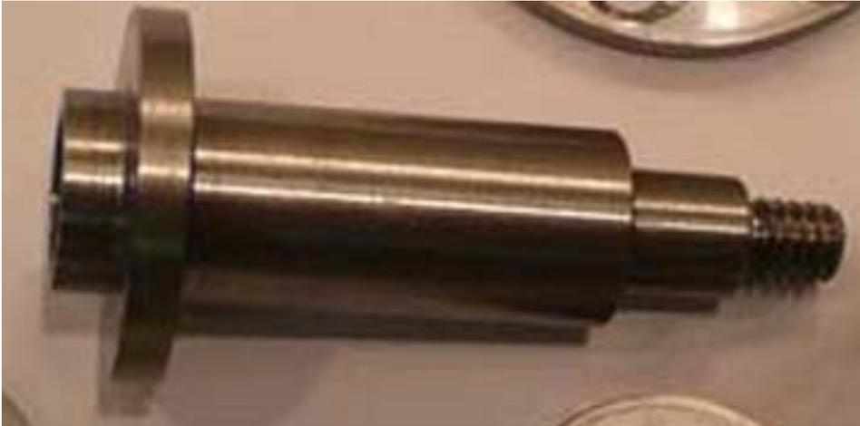
Figure 11 The Bearing Holder Insert.
