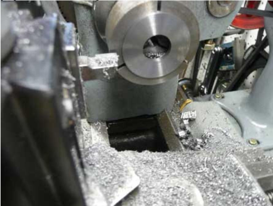
Figure 32 Facing the bearing retainer.
