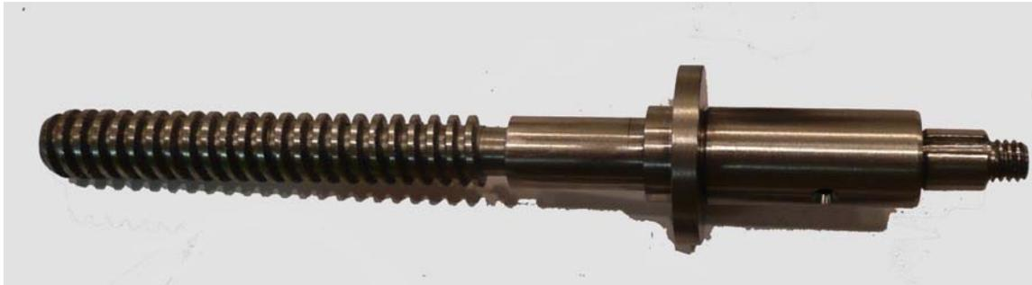
Figure 17 The completed compound screw and bearing block assembly.
