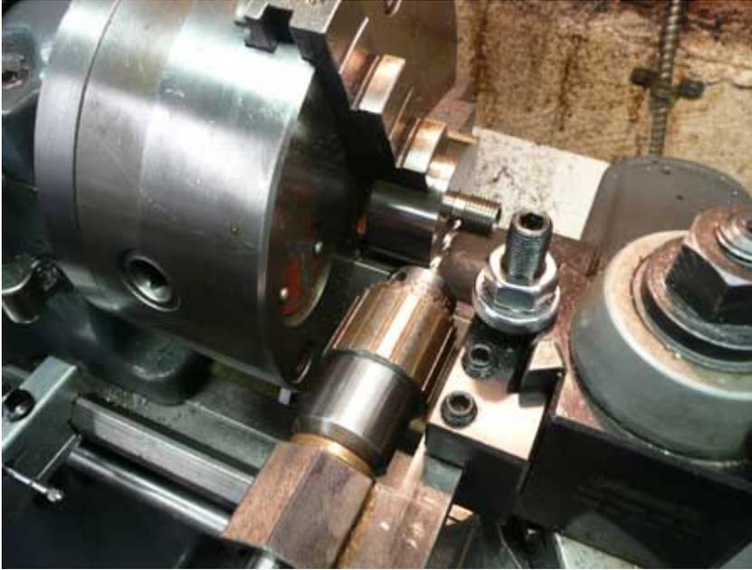
Figure 24 Cross drilling the Oil hole
