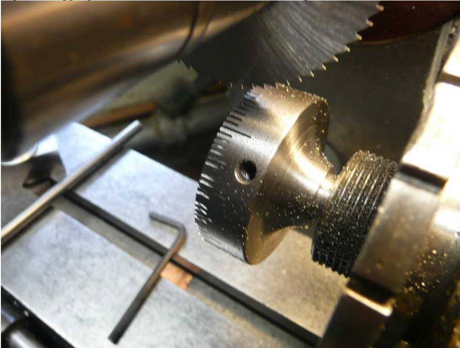
Figure 6 Marking the graduations. The dial is held in a collet and slot length are measured with a DI
