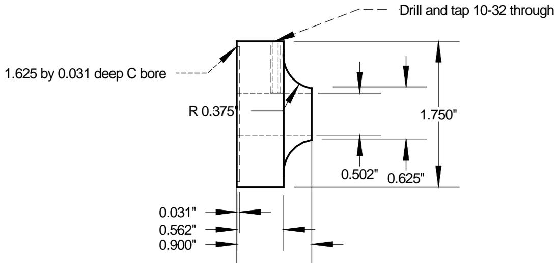
Figure 2 Dimensions for the Calibrated Dial
