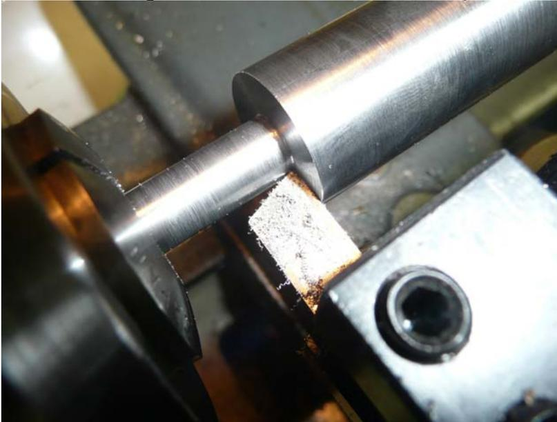
Figure 13 Removing tool radius and undercutting the diameter.
