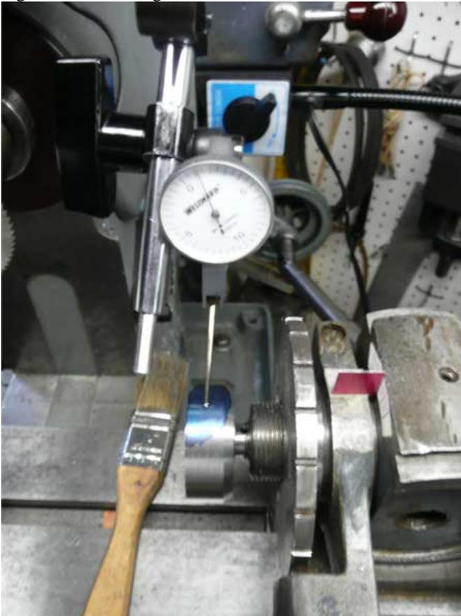
Figure 29 Setting the scribe line to TDC on the Mill
