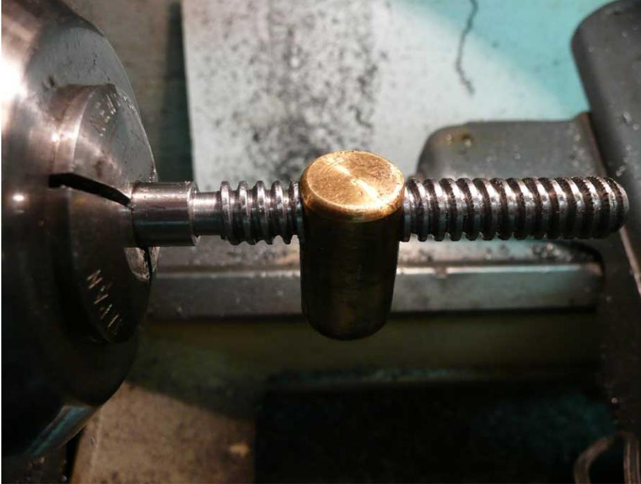
Figure 15 Compound nut on Shop made Acme Compound Screw.
