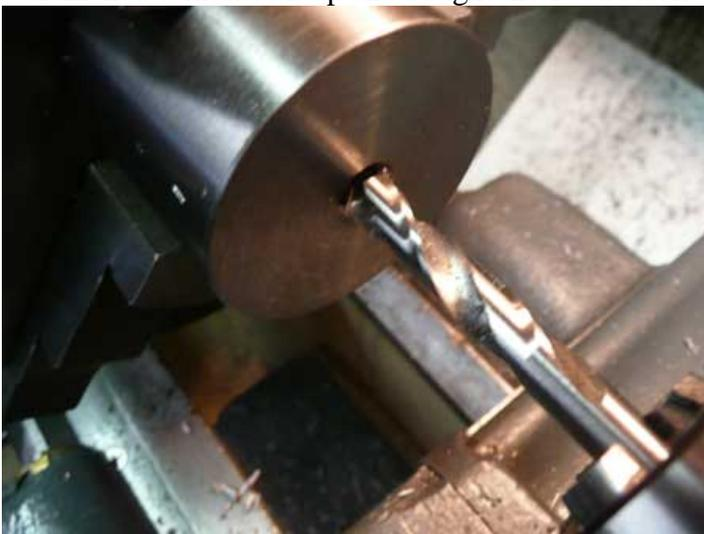
Figure 20 Drilling through the blank
