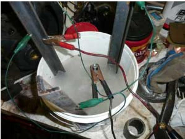
**Figure 19: Electrolytic tank**
