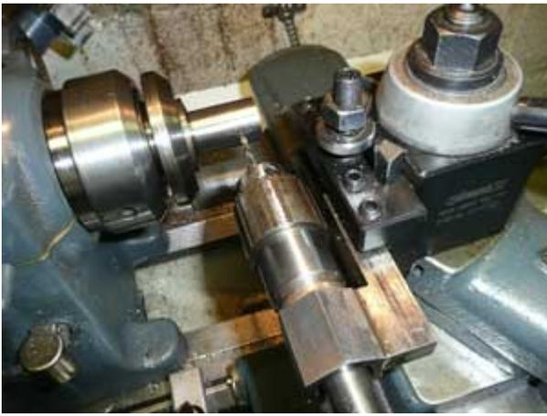
**Figure 17: Cross drilling weep hole**
