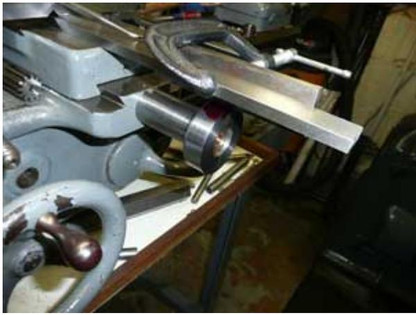
**Figure 12 Lining up the Zero Mark**
