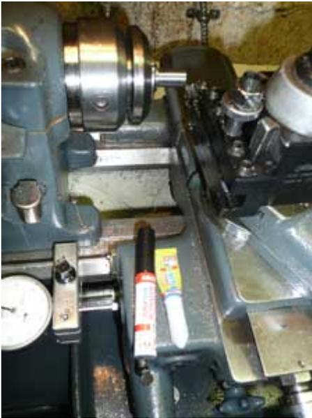
**Figure 23: With a 3/8" rod as support, Diameters turned.**
