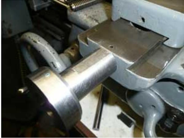
**Figure 15 The finished extension sleeve with markings and flat.**
