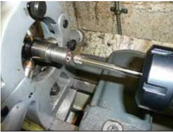
**Figure 10 Stub removed, bushing pressed, faced, and reamed.**
