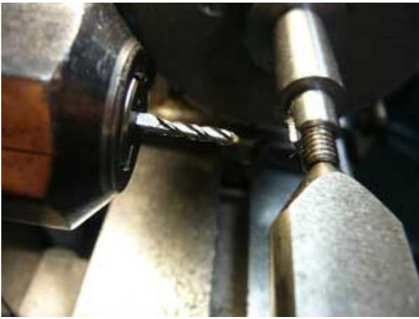
**Figure 22: Milling the Round bottom Key slot**
