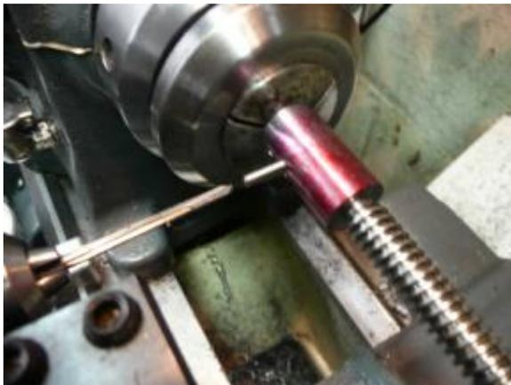
**Figure 21: Drill, ream and install taper pin**
