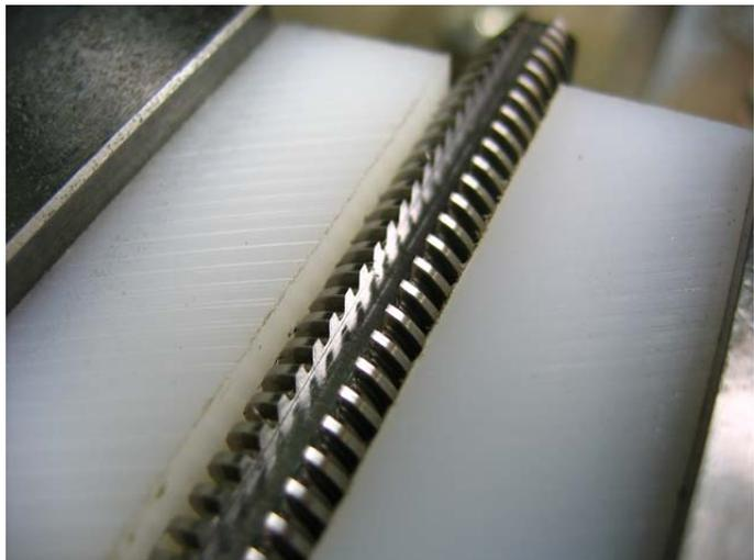
On the far end of the screw, I trimmed the 7/16" shoulder back so that a 5/16" ID thrust bearing behind the nut would bear up against the TA sleeve, not the screw and therefore allow the "slop" to be taken out of the leadscrew/TA sleeve. I replaced the Southbend nut with a metal locking nut so that just the right amount of preload could be put on the wavy spring washer without the nut backing itself off as the leadscrew turned.
