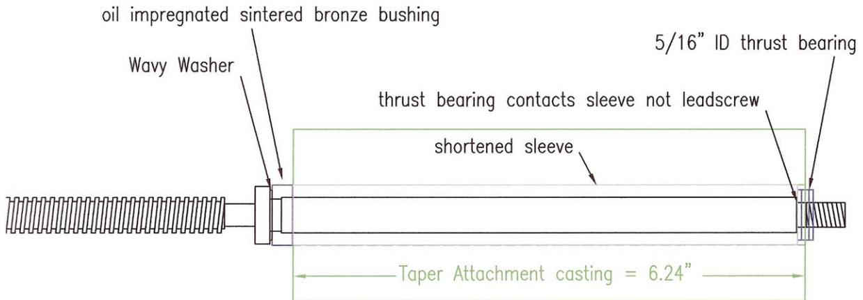
The handle assembly on the 10L is separate from the leadscrew. That is to say, the screw is driven by a key inside the gear shaft and is permitted to telescope in & out when using the taper attachment. However, the feel of the leadscrew assembly can be greatly improved by installing thrust bearings.
