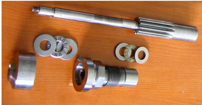
To fit the thrust bearings onto the handle assembly, the threaded crossfeed sleeve must be shortened at the small OD end and counterbored on the large OD end. The graduated dial must also be counterbored as the needle roller thrust bearing is centered between the two parts.
