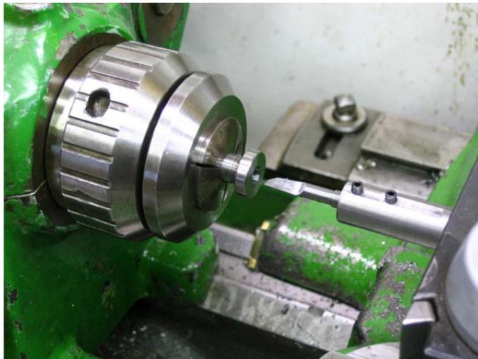
Turn down one end of the new acme screw to a diameter just under the size of the bore just made in the TA section. 0.279" x about 1.25" in my case. These figures are not critical. You just need a decent diameter to length ratio in order to get a good bond between the new screw and the old TA end. Keep the diameter as large as possible, but remove the acme threads entirely for maximum surface area contact.
