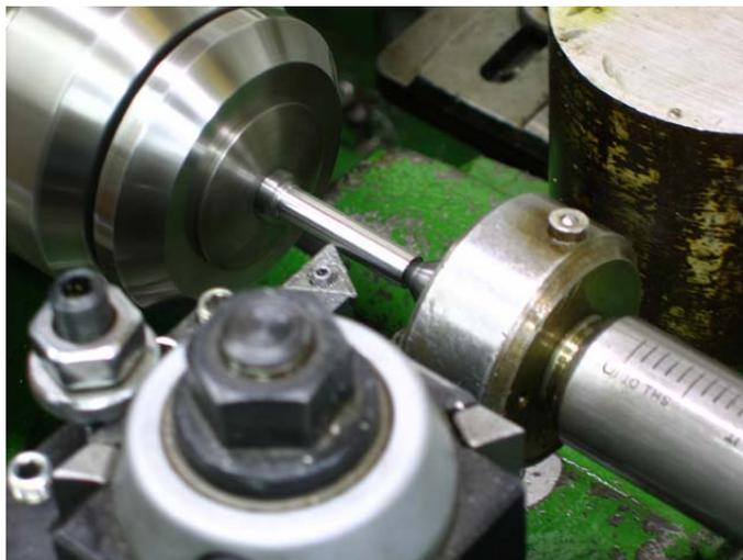
Dry fit the parts and measure their total length to determine what excess will need to be taken off the handle-end of the screw. Set the TA section aside and part off the calculated excess from the thread-end of the screw.
