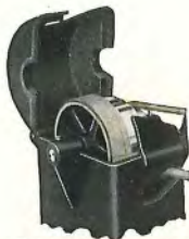
Cabinet Top Open Showing Drive Pulley
