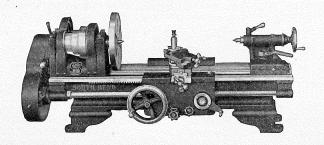
No. 27—11-IN. SOUTH BEND BENCH SCREW CUTTING ENGINE LATHE Fitted with Automatic Longitudinal Feed, Automatic Cross Feed and Graduated Compound Rest Regular equipment, as illustrated under Long Leg Lathe, is included in price of Bench Lathe
