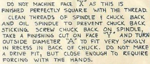
TO LOCATE HOLES IN CHUCK BACK, CHALK BACK OF CHUCK AND TAP CHUCK BACK LIGHTLY IN PLACE.
