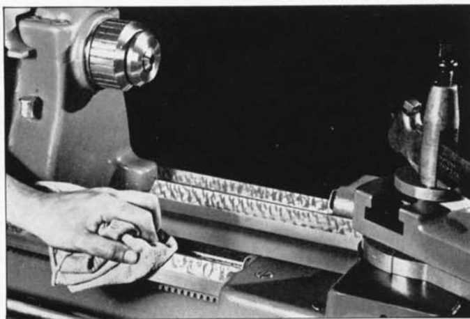
Fig. 5. A clean cloth can be used for removing the last traces of dust and grit.
