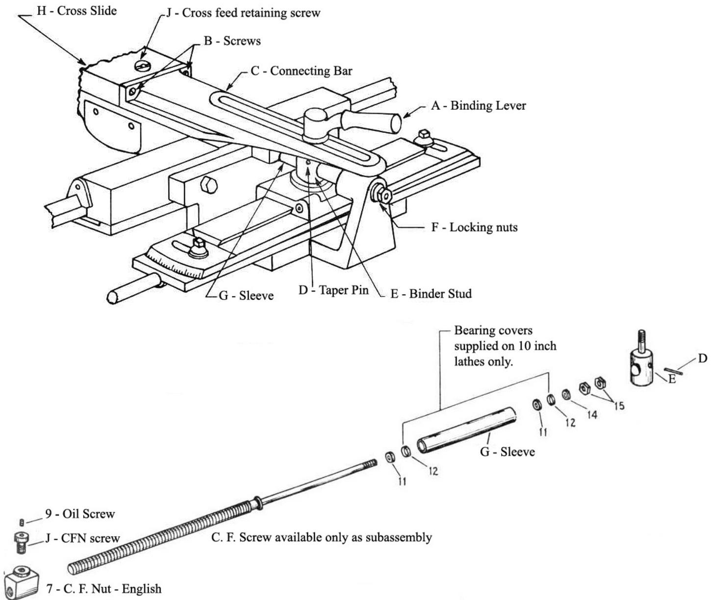
1. Remove Binding Lever "A" and collar.
