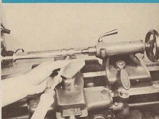
Carbide-tipped chisel curves curves as bored end of holder is supported by tailstock dead center with a brass plug turned to fit the hole snugly.
