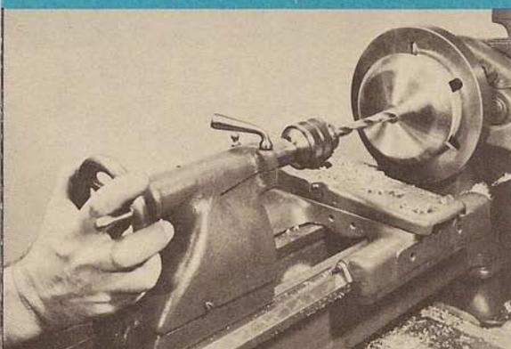
The center hole in the base is now made, but it must be tapped with a  $\frac{1}{2}$ -13 tap to accept the threaded end of the upright element of the unit.
