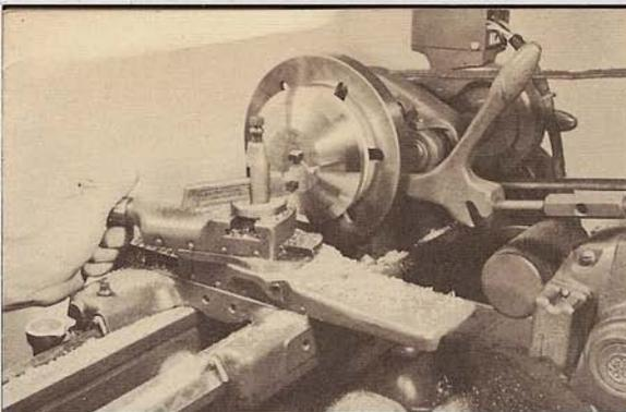
After base is rounded off, compound rest is set and base is roughly tapered. Although operation could be done with hand tool, this saves time.
